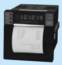
This instrumentation printer is designed for instrumentation amplifiers WGA-650B/670B/710B/800C. With the thermal serial dot matrix system, it prints out parallel BCD data, 24 characters per line. Besides 14 kinds of messages, the built-in calendar clock enables printout of the date, time and elapsed time as well as interval print in a range of 5 seconds to 99 hours 59 minute 59 seconds. (Note that the printer is different from Tsuruga Micro Printer 442B.)
